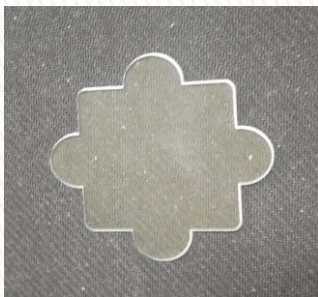
Glass Cutting wavelength: 355nm
