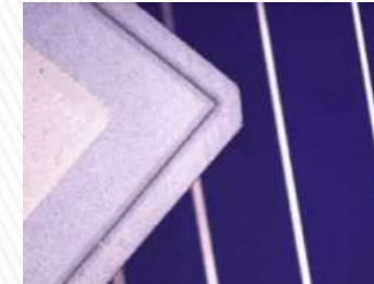
Edge Isolation of Si Solarcell Wavelength: 1064nm Pulse energy: Rep rate: 500kHz Proceeding speed : 2m/s
