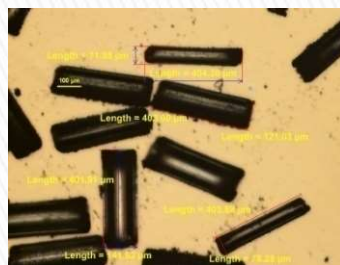
Glass Microwire Cutting Wavelength: 355nm
