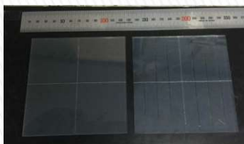
FTO Scribing Wavelength: 532nm
