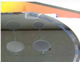
Si Wafer Drilling Wavelength : 532nm
