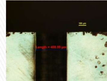
Diamond Pattern Scribing wavelength: 532nm
