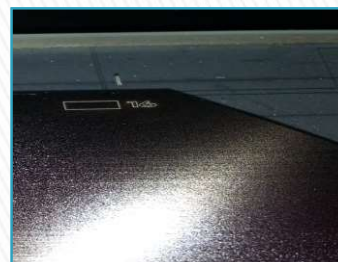
Si Wafer Align Key Marking Wavelength: 355nm
