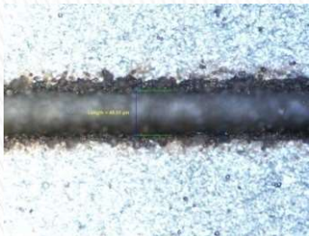
LGBC Scribing (Laser Grooved Buried Contracts) Wavelength: 355nm
