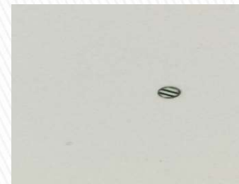
Ceramic Cutting (Ni Oxide + YSZ) Wavelength: 1064nm
