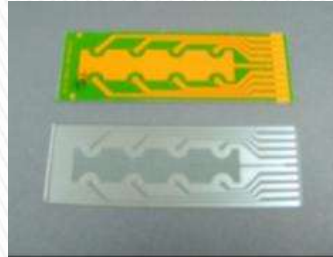
FTO Patterning (FTO on glass) Wavelength: 1060nm
