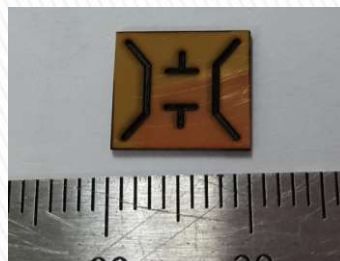
Sapphire Wafer Cutting (Cross-Section) Wavelength: 355nm
