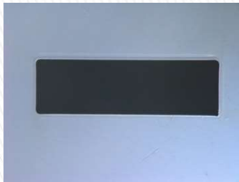
PMMA Cutting Wavelength: 10.6 \mu\text{m}
