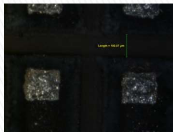
Aluminium Through Line Patterning Wavelength: 532nm
