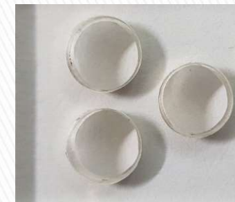
PC Hole Drilling Wavelength: 355nm Thickness: 4mm
