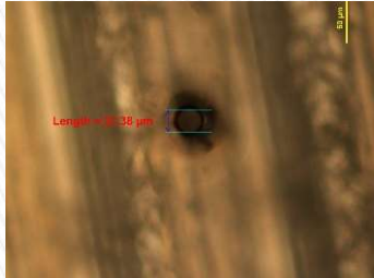
Glass Hole Drilling Pico 355 UV Thickness: 30μm Diameter: 21 μm
