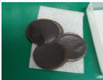
Graphene Cutting Wavelength: 355nm
