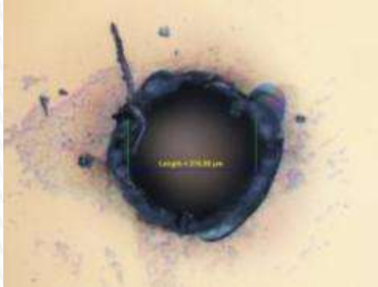
Via Hole Wavelength: 355nm
