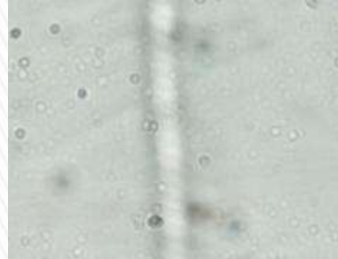
Scribing of Glass Wavelength: 532nm Pulse energy: Rep rate: 30kHz Proceeding speed : 200mm/s
