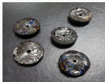
Carbon Disk Hole Drilling (100% Carbon) Wavelength: 355nm
