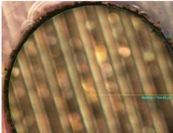
PET Film Cutting Wavelength: 355nm
