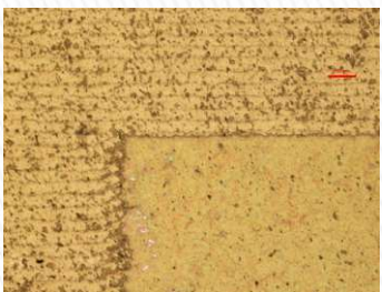
Si Wafer Hatching Patterning Wavelength: 355nm
