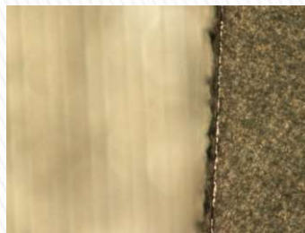
Ceramic Cutting (Ni Oxide + YSZ) Wavelength: 1064nm
