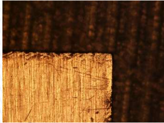
SUS Cutting Wavelength: 355nm Thickness: 0.1mm
