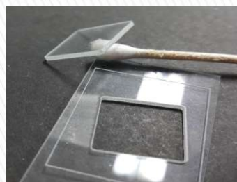
Slide Glass Cutting Wavelength: 355nm
