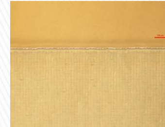
FTO Release (FTO on glass) Wavelength: 355nm
