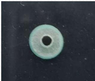
Glass Hole Drilling wavelength: 355nm Thickness: 4mm
