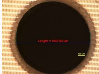
LCD(2 Layers) Hole Cutting Pico 355 UV Thickness: 300μm Diameter: 1mm
