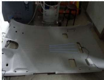
Epoxy Resin Patterning Wavelength: 10.6μm
