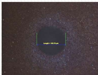
Fired Ceramic Sheet (Via Hole) Wavelength: 355nm
