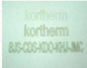
Glass Patterning Wavelength: 355nm
