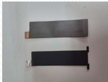
Cathode/Anode Electrode Cutting (Copper & Aluminium) Wavelength: 355nm Thickness: 25μm
