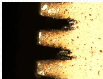
Si Wafer Patterning Wavelength: 532nm
