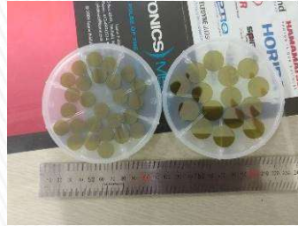
Sic Wafer Cutting Wavelength: 355nm Thickness: 0.6mm
