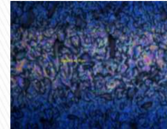
Solar cell Wafer Edge isolation Wavelength : 532nm
