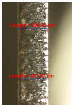
Si Wafer Hatching Patterning Wavelength: 355nm
