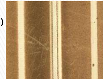
Removing of ZnO on Glass Wavelength: 355nm Pulse energy: Rep rate: 30kHz Proceeding speed : 200mm/s
