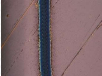
Perovskite Scribing Pico 355 UV Thickness: 30 \mu m
