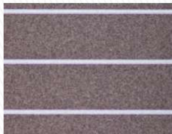
Removal of TCO on CIGS + Mo+Glass Wavelength: 1064nm Pulse energy: Rep rate: 500kHz Proceeding speed : 2m/s
