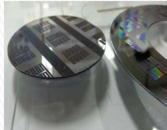
Si Wafer Round Cutting Wavelength: 532nm Thickness: 520 \mu\text{m}
