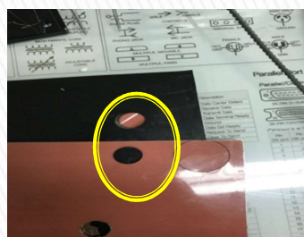
OLED Light Hole Drilling Wavelength: 355nm Thickness: 0.88mm
