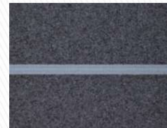
Removal of CIGS on Mo+Glass Wavelength: 1064nm Pulse energy: Rep rate: 500kHz Proceeding speed : 2m/s
