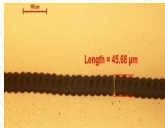
Mo Scribing (Solar Cell Thin Film) Wavelength: 532nm
