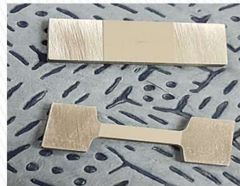
Cathode/Anode Electrode Cutting (Copper & Aluminium) Wavelength: 355nm Thickness: 25μm
