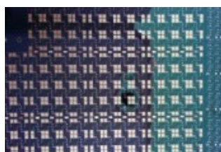
Si Wafer Pattern Cutting Wavelength : 532nm
