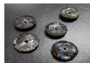
Carbon Disk Hole Drilling (100% Carbon) Wavelength : 355nm
