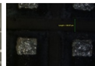
Aluminium Through Line Patterning Wavelength : 532nm
