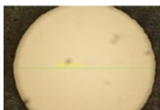
Drilling of Si-Wafer Wavelength : 1064nm Pulse energy : Rep rate : 10kHz
