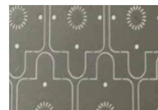
SUS304 Hole Drilling Wavelength : 355nm
