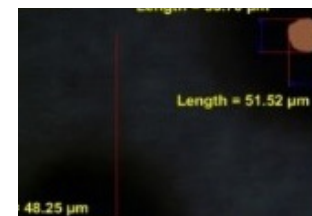
Cu Hole Drilling Wavelength: 355nm Thickness : 0.1mm
