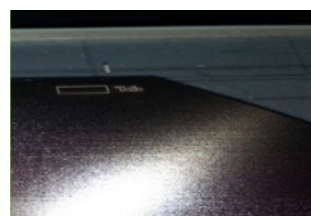
Si Wafer Align Key Marking Wavelength : 355nm
