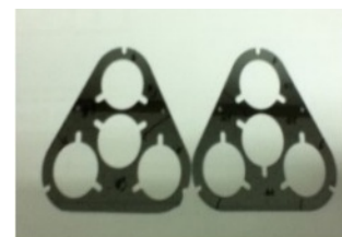
Si Wafer Pattern Cutting Wavelength : 532nm
