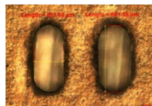
Silicone Sheet Hole Drilling Wavelength : 355nm
