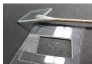
Slide Glass Cutting Wavelength : 355nm
