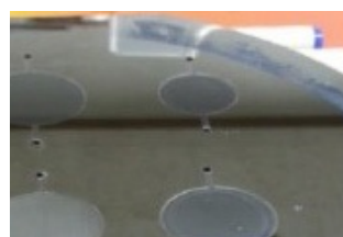
Si Wafer Drilling Wavelength : 532nm
