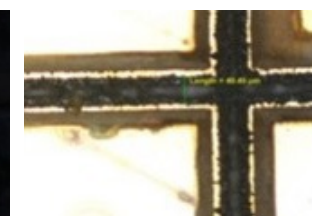
Metal Oxide Film Ablation Wavelength : 532nm
