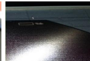
**Si Wafer Align Key Marking**
